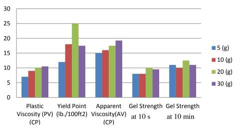
Figure 8. Rheology properties of 10% bentonite mud with rice husk ash.
