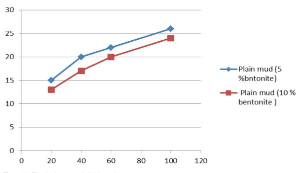
Figure 13. Filtration loss control of plain mud.
