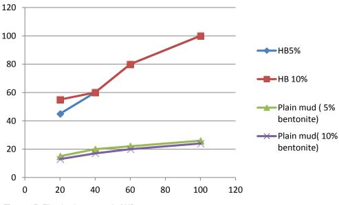
Figure 15. Filtration loss control of HB.
