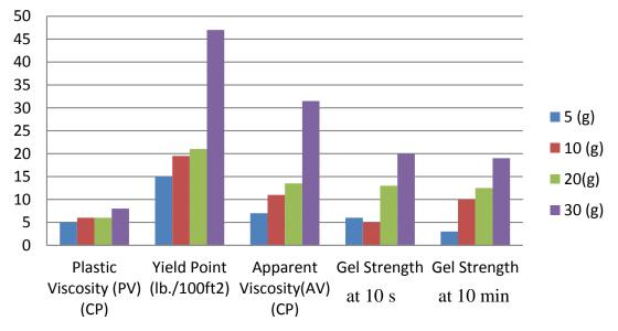
Figure 10. Rheology properties of 10% bentonite mud with hay barn.
