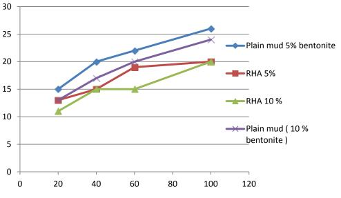
Figure 14. Filtration loss control of RHA.
