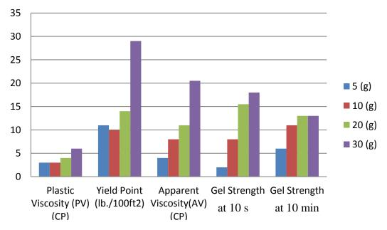
Figure 12. Rheology properties of 10% bentonite mud with hay barn ash.
