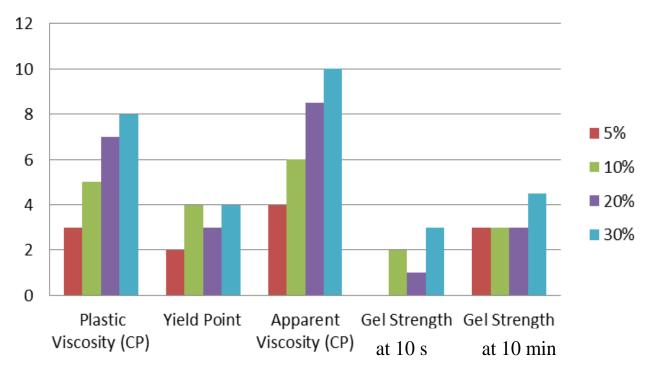
Figure 7. Rheology properties of 5% bentonite mud with rice husk ash.
