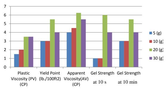
Figure 11. Rheology properties of 5% bentonite mud with hay barn ash.
